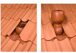
**ENG:** Then set all the tiles into place. You may have to cut off a piece from the bottom of some tiles, so that the tile sits evenly against the batten. Check with a builder's level that the pipe is vertical. Mount the pipes to the pass-through with six screws.
