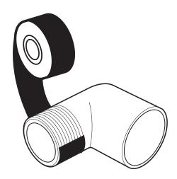
**2** Attach elbow with 3/4" slip &3/4"G to the primary drain connection.
