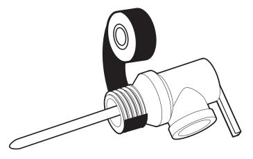
2 Install the T&P relief valve in the opening marked T&P relief valve.
