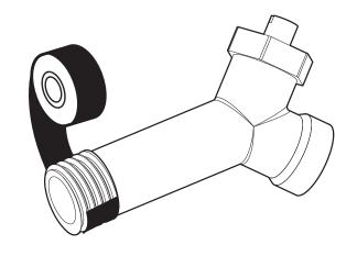
2 Install the drain valve in the opening marked "Drain Valve".
