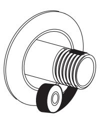
Connect cold and hot water supply using 3/4" G.
