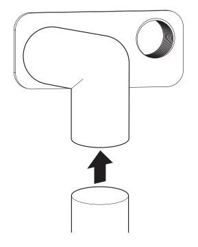
**4** Using 1/2" PVC piping, an elbow with 1/2" slip & 1/2" G, and an approved sealant, attach the elbow to secondary drain connection and insert the PVC pipe into the female end.
