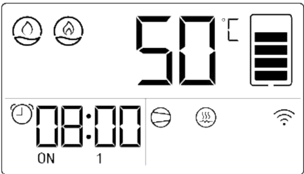
Fig. 5-3 Turn on BOOST mode
