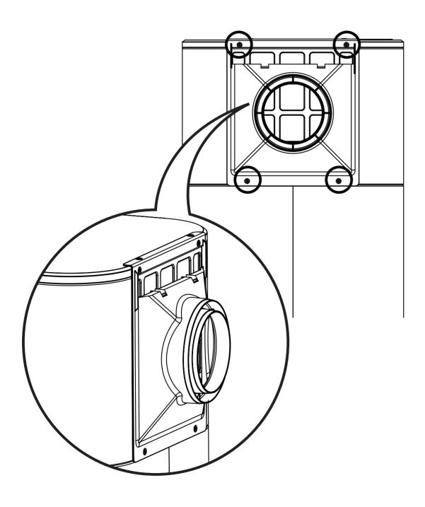
3 Assemble the duct cover with guiding ribs.
