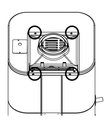
4 Assemble the duct cover with guiding ribs.
