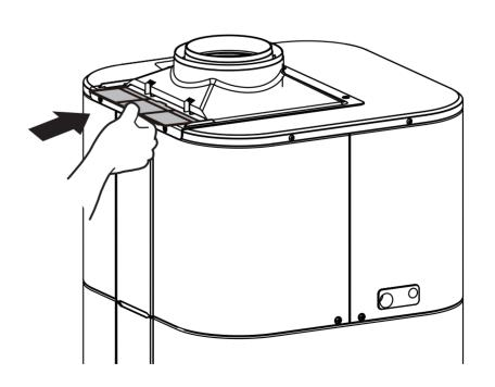
**7** Assemble the duct cover with guiding ribs.
