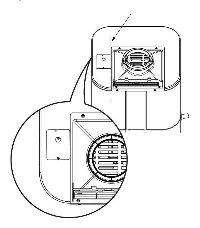
**3** Fasten it with additional screws in the installation box.
