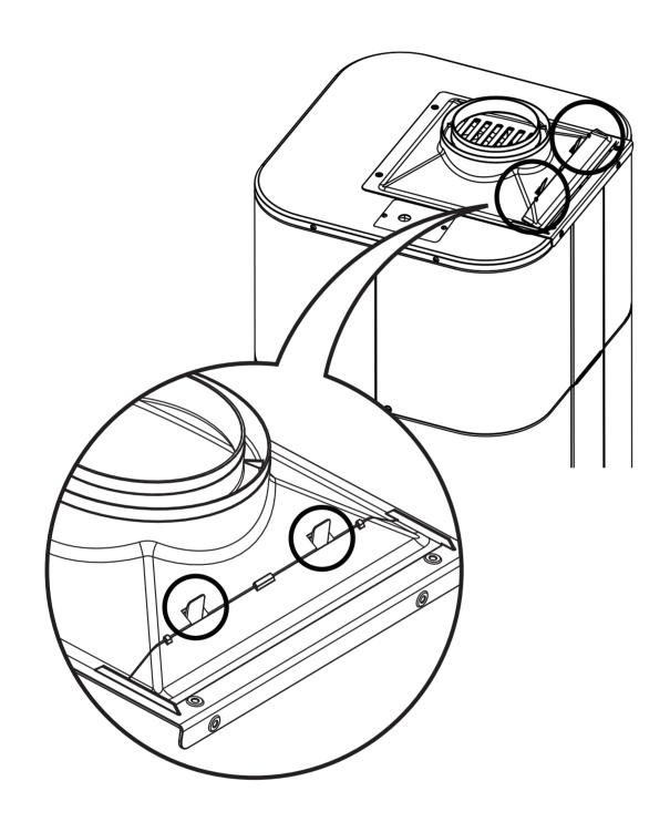
3 Hold the knobs of the air filter, pull out the filter from the top cover.
