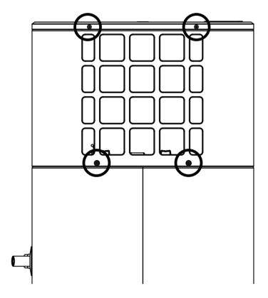
2 Place the duct adaptor and align the each holes and fasten it with additional screws in the installation box.
