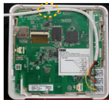
The Upper center boss for fixing the bent cable
